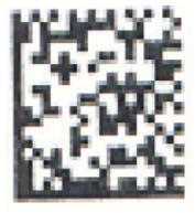
150 dpi uncompressed. Higher resolution results in much sharper definition of barcode elements.
